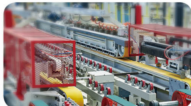
★ NDMBZH 系列机型采用伺服推砖系统，可选配对角线自动调整装置。 NDMBZH series machine using brick pushing system and diagonal automatic adjustment device is optional.
